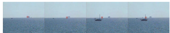
Fig. 18 The KLT feature tracker is far too sensitive to the partial occlusion. It cannot track the desired target.
