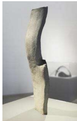
Figure 3. Test Piece, 1.2 mm high/24 cm wide doubly curved composite shell
