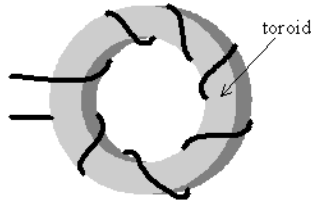
Figure 5.12: An inductor with 7-turn solenoidal wound conductor.
